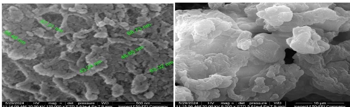
Fig1: FESEM microimage of Nano polystyrene (500nm and 10 $\mu\text{m}$ )
