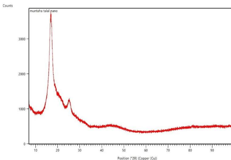
**Fig 5:** XRD of the Nano-Polystyrene.
