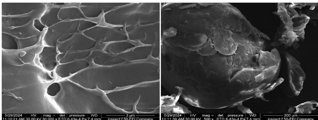
**Fig 2:** FESEM microimage of polystyrene (3 μm and 200μm)
