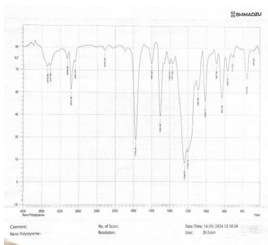
**Fig.4:** FTIR of Nano polystyrene material
