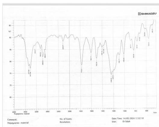
**Fig.3:** FTIR of polystyrene material
