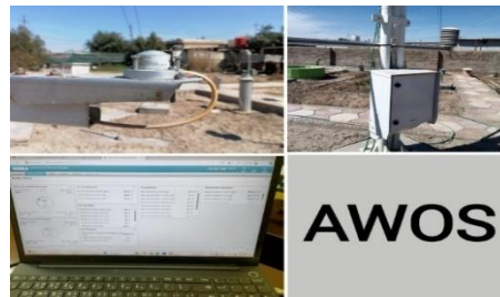
Fig. 11. Shows the AWOS system for measuring atmospheric elements and solar radiation
