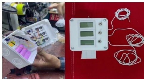
Fig. 10. Shows the electronic thermometer used to measure temperature
