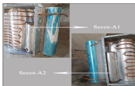
Fig.5. Shows the location of the two tanks installed inside the Scccs1
